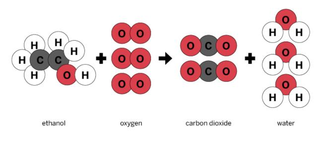
When ethanol burns, it mixes with oxygen, and the atoms of these reactants rearrange to form two products: carbon dioxide and water in the gas phase.
